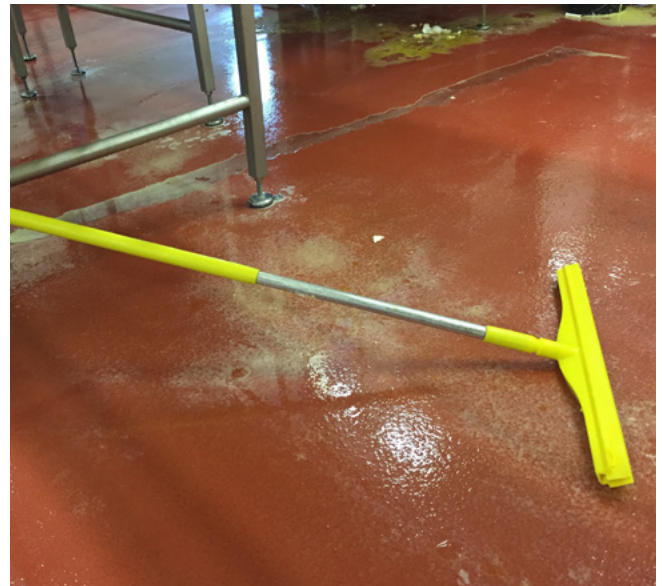
Squeegee that can be used instead of hoses to wash floors.
